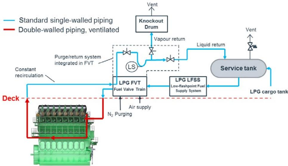
Figure 11: Schematic diagram of engine, fuel service tank and piping. Source: MAN
