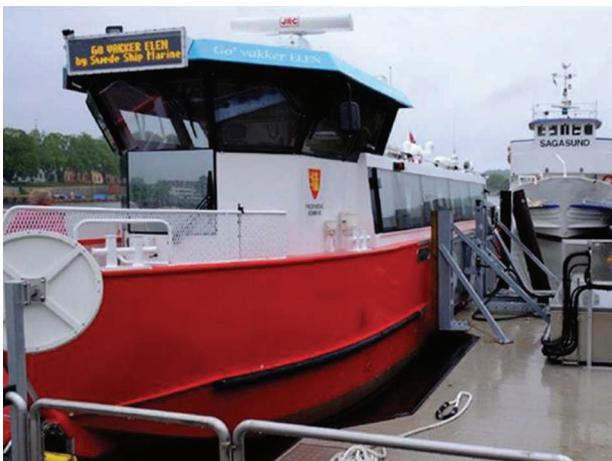
Figure 14. Inductive shore-to-ship charging for the Go Vakker Elen shuttle ferry. (Source: Swede Ship Marine; used with permission.)
