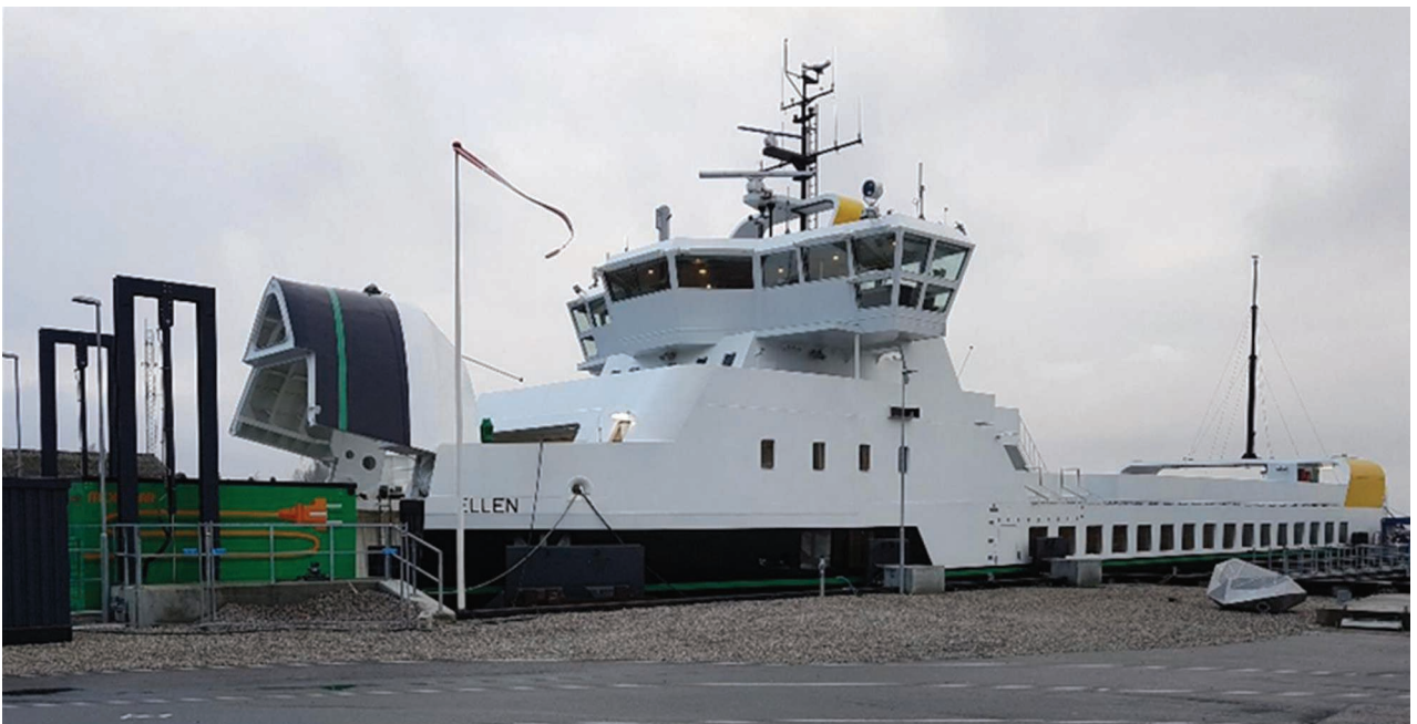
Figure 10. The Mobimar Nectors dc-based charging station for the E-ferry Ellen . (Source: Mobimar; used with permission.)
