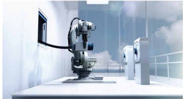
Figure 7. The ABB IRB7600, an autonomous robotic arm used for charging the MS Aurora and MF Tycho Brahe . (Source: ABB; used with permission.)
